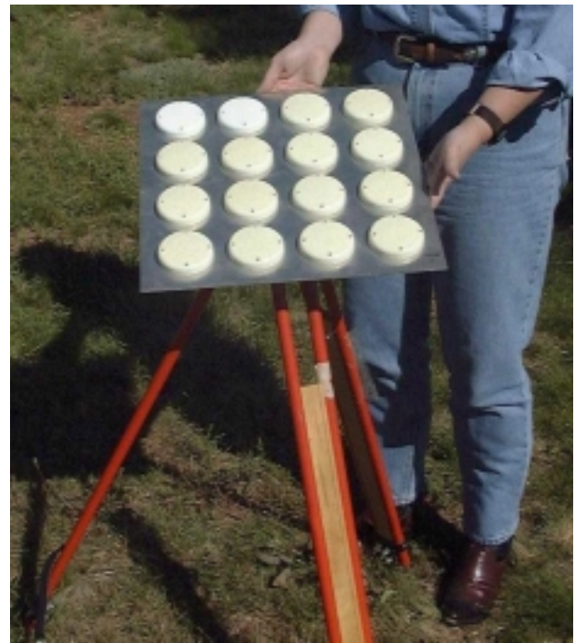
Figure 6 HAGR 16-element antenna array
