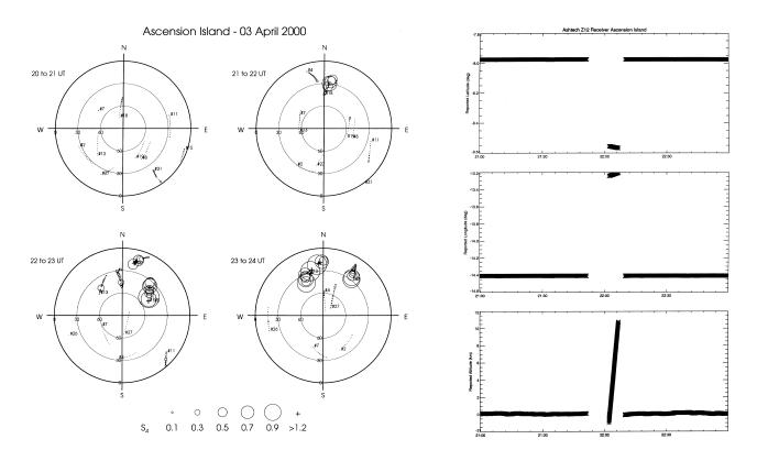
Figure 8 a) Hourly polar plots of the position and scintillation levels, plotted at 5 min intervals, of all GPS links tracked by the ISM at Ascension Island, 4 April 2000. Circle size corresponds to S4 level as shown in the legend. PRN numbers are plotted at the initial satellite position; b) Corresponding position data reported by the Ashtech Z-12
