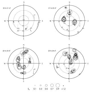
Figure 2. Hourly polar plots of the position and scintillation levels, plotted at 5 min intervals, of all GPS links tracked by the Ionospheric Scintillation Monitor at Ascension Island, 27 March 2000. Circle size corresponds to S4 level as shown in the legend. PRN numbers are plotted at the initial satellite position.
