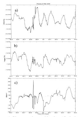
Figure 4. Plessey receiver position data a) Latitude, b) Longitude and c) Altitude.
