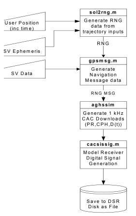
Figure 5 AGHS MATLAB Signal Simulation
