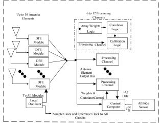
Figure 6 P(Y) HAGR System Block Diagram
