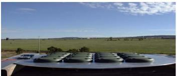
Figure 2 Sixteen Element L1/L2 Antenna Array
