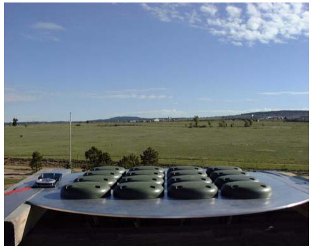
Figure 5 Sixteen Element HAGR Antenna Array
