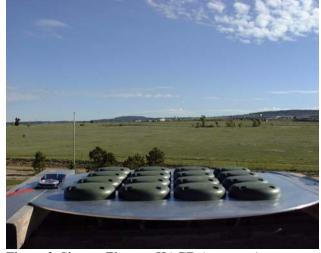
Figure 2 Sixteen Element HAGR Antenna Array
