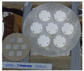
Figure 3 Seven-Element CRPA and Mini-Array
