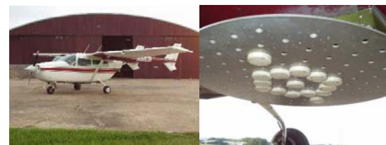
Figure 13 Cessna Test Aircraft and Antenna Array Mounted underneath
