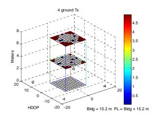
Figure 6 HDOP with 4 Ground-Based Transmitters
