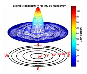
Figure 8 Beam Pattern of 109-Element Array
