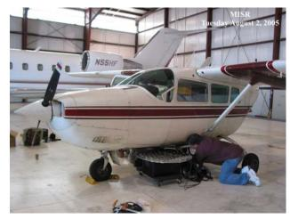
**Figure 4 96 Element Antenna Array Installation**
