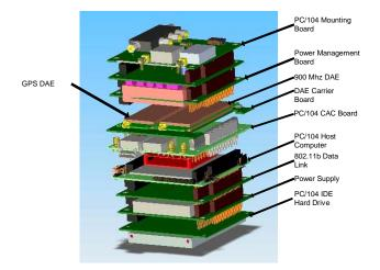
Figure 3 POSCOMM SDR Components
