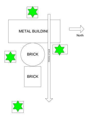
Figure 9 Indoor Test Pseudolite Layout
