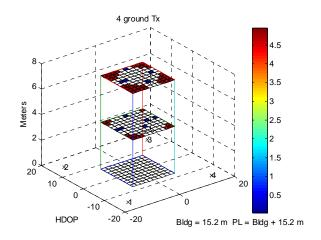
Figure 6 HDOP with 4 Ground-Based Transmitters
