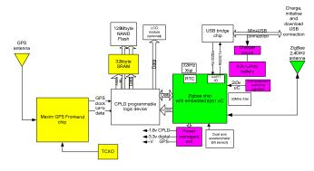
Figure 4 GeoZigBee Device Components
