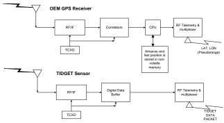
Figure 2 TIDGET Sensor
