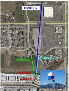
Figure 3 Extended Range ZigBee Connection
