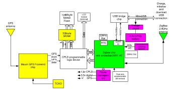
Figure 4 GeoZigBee Device Components
