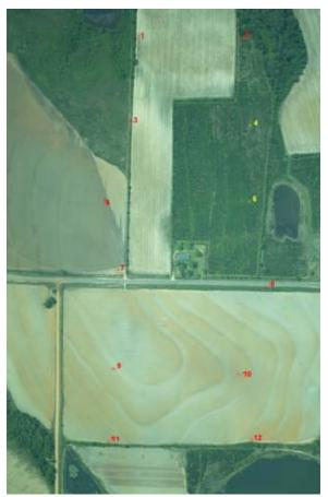
Figure 16 Actual GCPs located automatically
