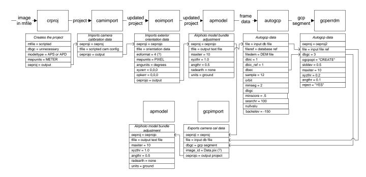
Figure 6 Image bundle adjustment data flow
