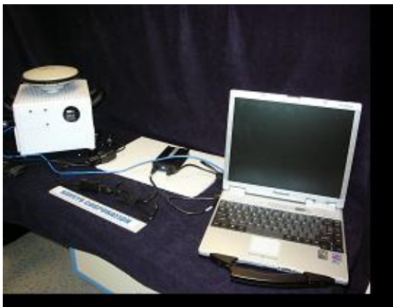
NGA Tactical Surveying and Targeting System (TS2)
