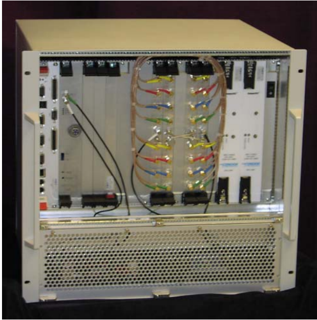
Figure 2 16-Element L1 Only Rack-Mounted SSGR
