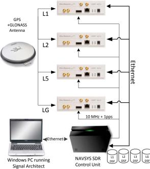
Figure 10 Future Multi-Frequency GNSS Signal Generator Configuration
