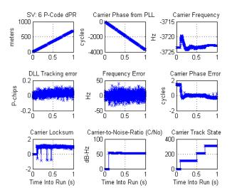
Figure 6 P-Code Tracking Results
