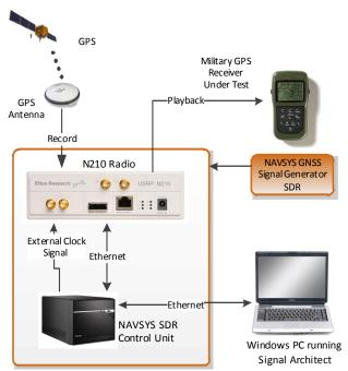
Figure 3 NAVSYS GNSS Signal Generator Hardware
