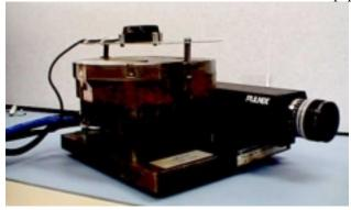
Figure 2 GPS/Inertial/Video Sensor Assembly
