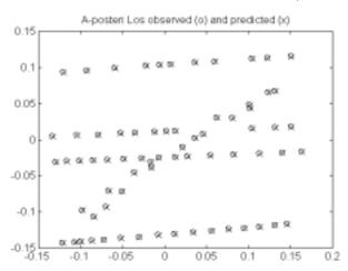
Figure 5 Post Calibration Pixel Coordinate Errors (~0.3 mrad RMS)
