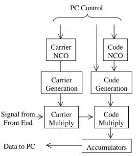
**Figure 5 Correlator Accelerator Card Functions**
