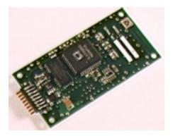
**Figure 4 TIDGET Digital Front End**
