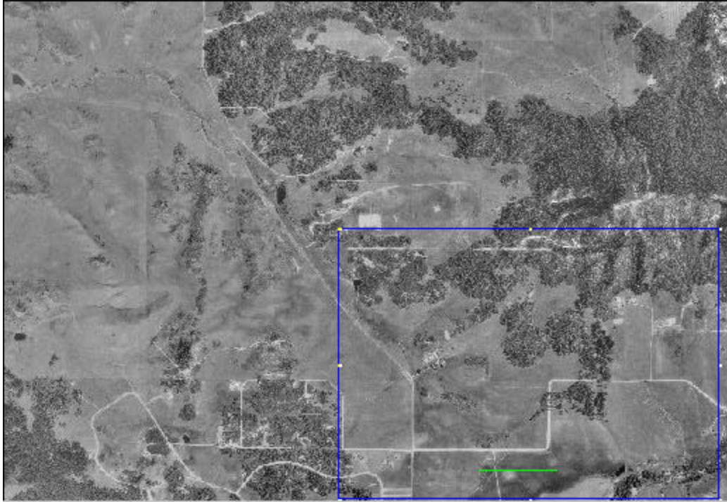
Figure 12 Input image with feature found within the search region using cross-correlation
